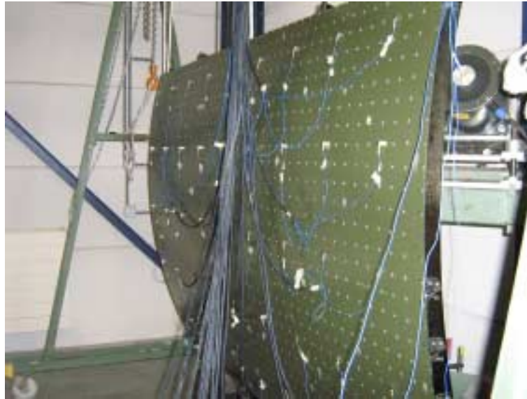
Figure 1 Front view of the composite fuselage panel mounted in the test rig
