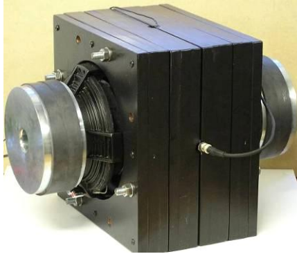
Figure 4. High sound level particle velocity calibration
