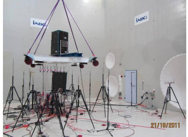
Figure 5. Setup with all probes, arrays and test articles
