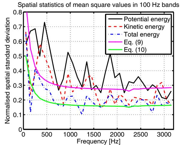
Fig. 3. Normalised spatial standard deviation of potential, kinetic and total energy density in 100 Hz bands.
