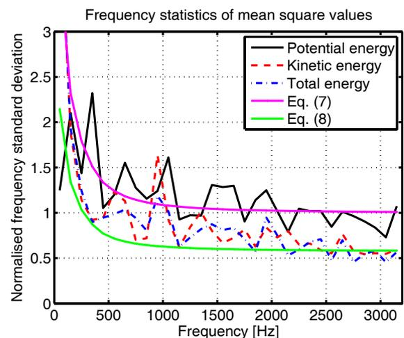
Fig. 4. Normalised standard deviation of potential, kinetic and total energy density with respect to frequency at one single position, calculated in 100 Hz bands.
