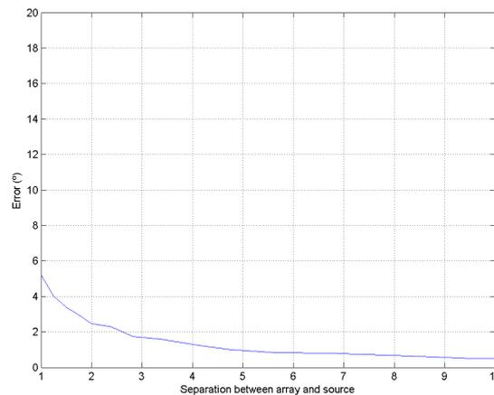
**Figure 2.** MUSIC positional error after synthesize the spectral matrix for different separation distance  $r_n$
