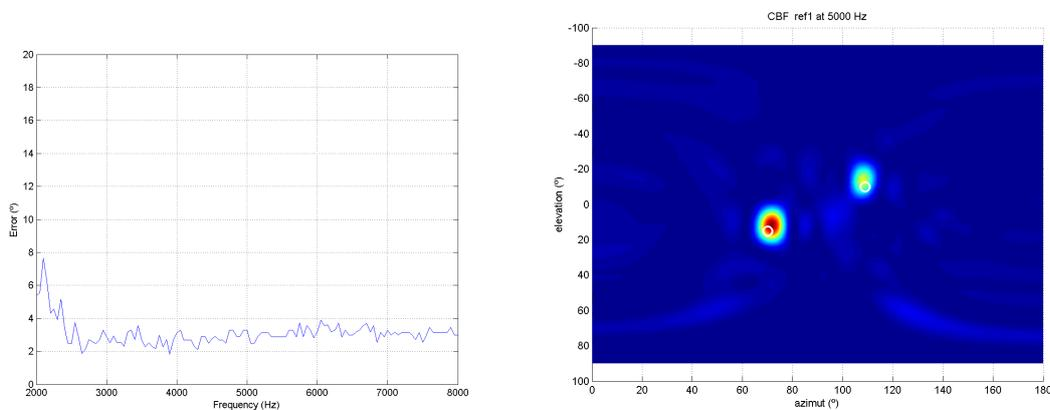
**Figure 3.** CBF error across the spectrum (left) and CBF localization map at 5 kHz (right)
