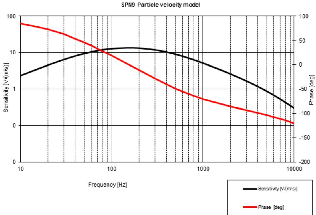
Figure 3. Typical SPN9 Microflown response model
