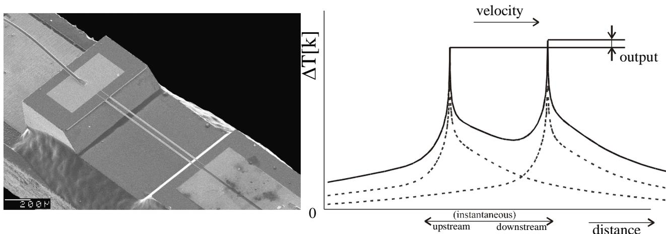
Figure 1. Sensor principle
