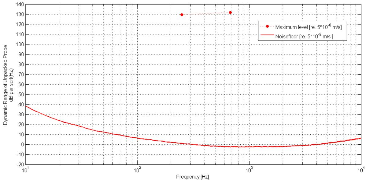
Figure 2. SPN0 probe and MFPA-1 dynamic range
