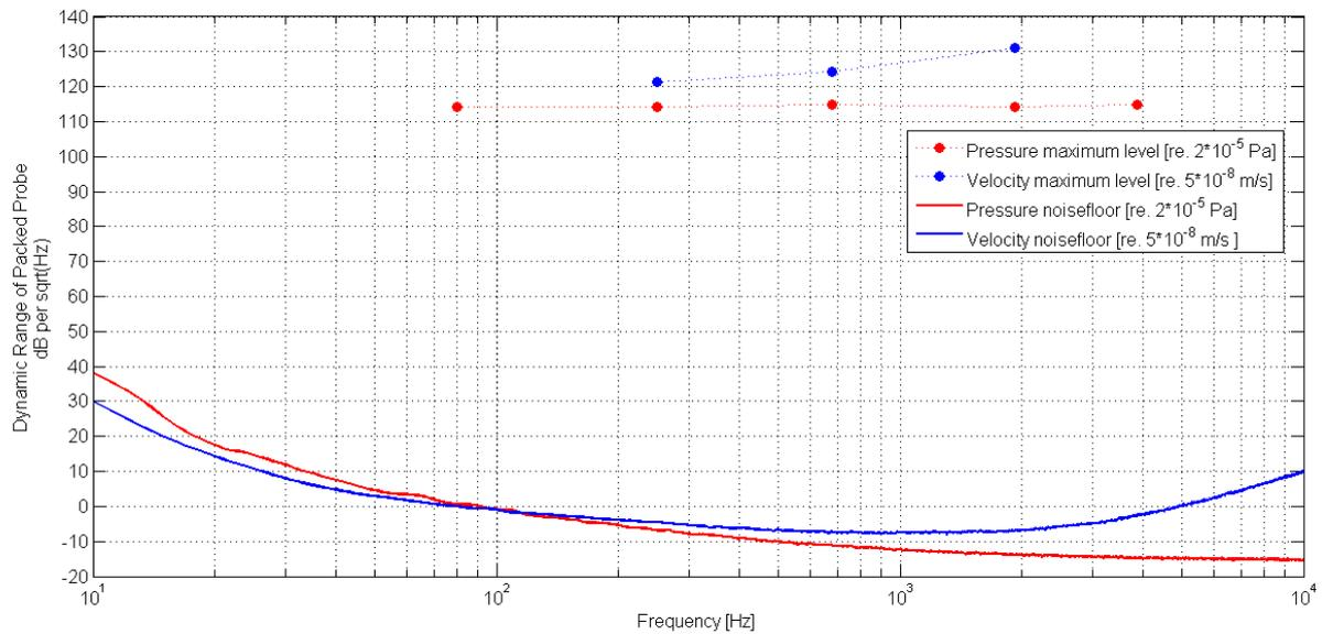
Figure 2. PR probe and MFPA-2 dynamic range
