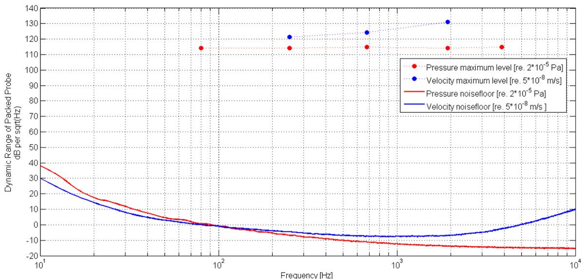
Figure 2. PM probe and MFPA-2 dynamic range
