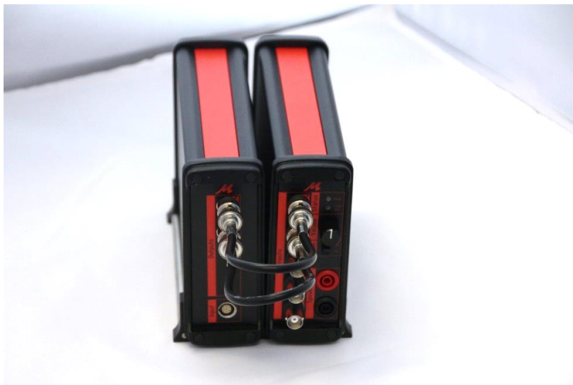
Figure 2. Connect MFPA to Frontend with as many BNC cables as MFPA outputs
