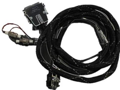
Figure 2. BNC connectors on 50 Pin Universal cable to Reference sensors
