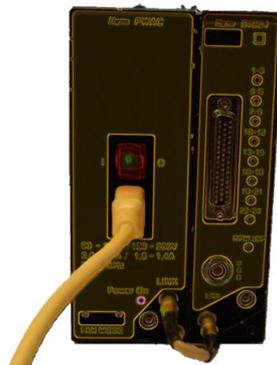
Figure 5. Connect power cable and link PWAC-DIC24; Click power ON.
