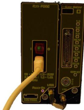
Figure 5. Connect power cable and link PWAC-DIC24; Click power ON.
