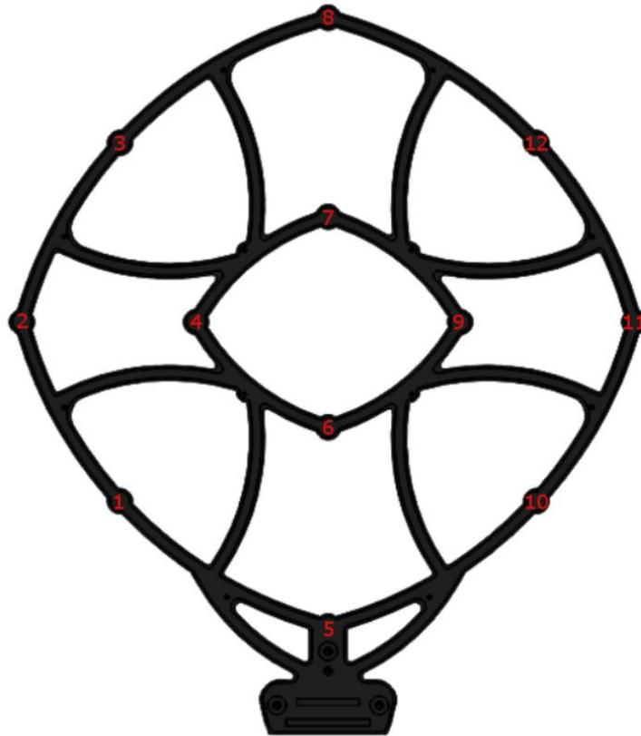
Follow the probes connection diagram above in order to match the calibration values with the proper channel input in the software.
