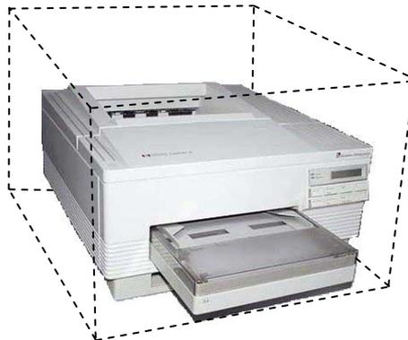
Figure 8: Printer with indicated partial measurement areas
